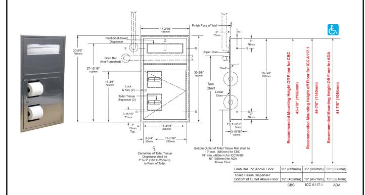
**Note:** For accessible toilet compartments, please use horizontal recessed or surface -mounted combination dispenser-/disposal-units, B-3091 or B-3092 Series, to comply with ADA 1-1/2" absolute Grab Bar wall spacing.
