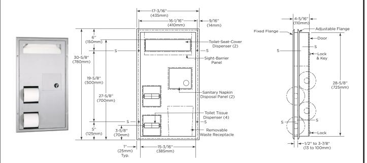
**Note:** For accessible toilet compartments, please use horizontal recessed or surface -mounted combination dispenser-/disposal-units, B-3091 or B-3092 Series, to comply with ADA 1-1/2" absolute Grab Bar wall spacing.
